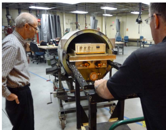
During a test phase for the PODEX experiment, engineers and the crew at Dryden Aircraft Operations Facility loaded the Research Scanning Polarimeter into the "superpod," for placement under the wing of the ER-2. Image credit: NASA/Matteo Ottaviani
